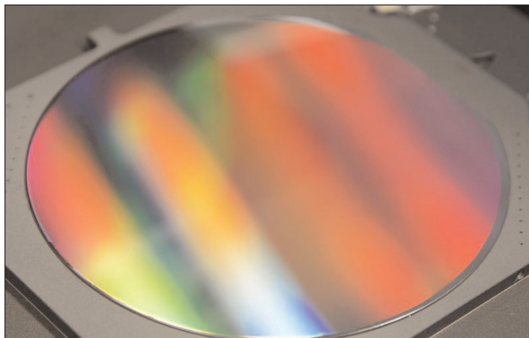
A 6-inch full-area nanoimprinted wafer processed by EVG NIL solutions.
