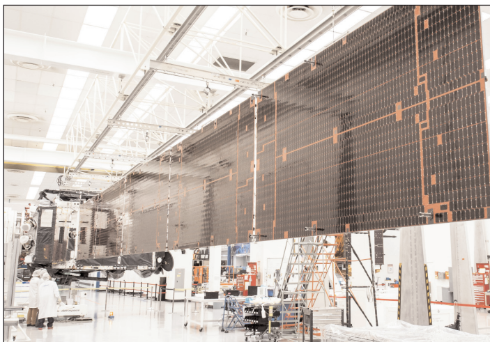
A satellite in Boeing's Satellite Development Center in El Segundo, powered by solar panels built by Spectrolab.
