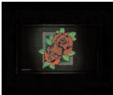
The first single-panel, full-color micro-display suitable for AR applications, based on Porotech's Dynamic Pixel Tuning technology.
