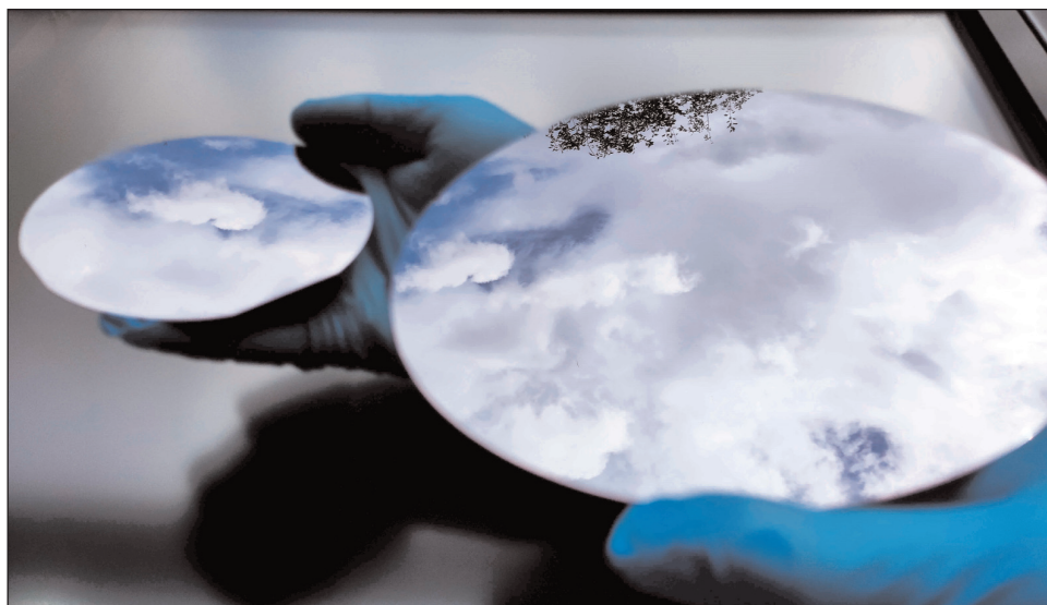
InP-on-GaAs substrates with 100mm and 150mm diameter, which can be used as a direct replacement for classical InP substrates. (© Fraunhofer ISE/photo: Carmine Pellegrino.)
