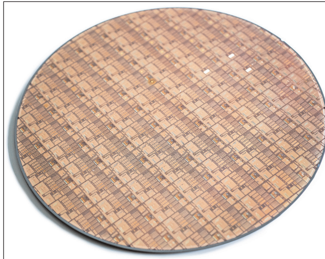
imec's 325GHz RF silicon interposer platform for advanced chiplet-based heterogeneous systems.
