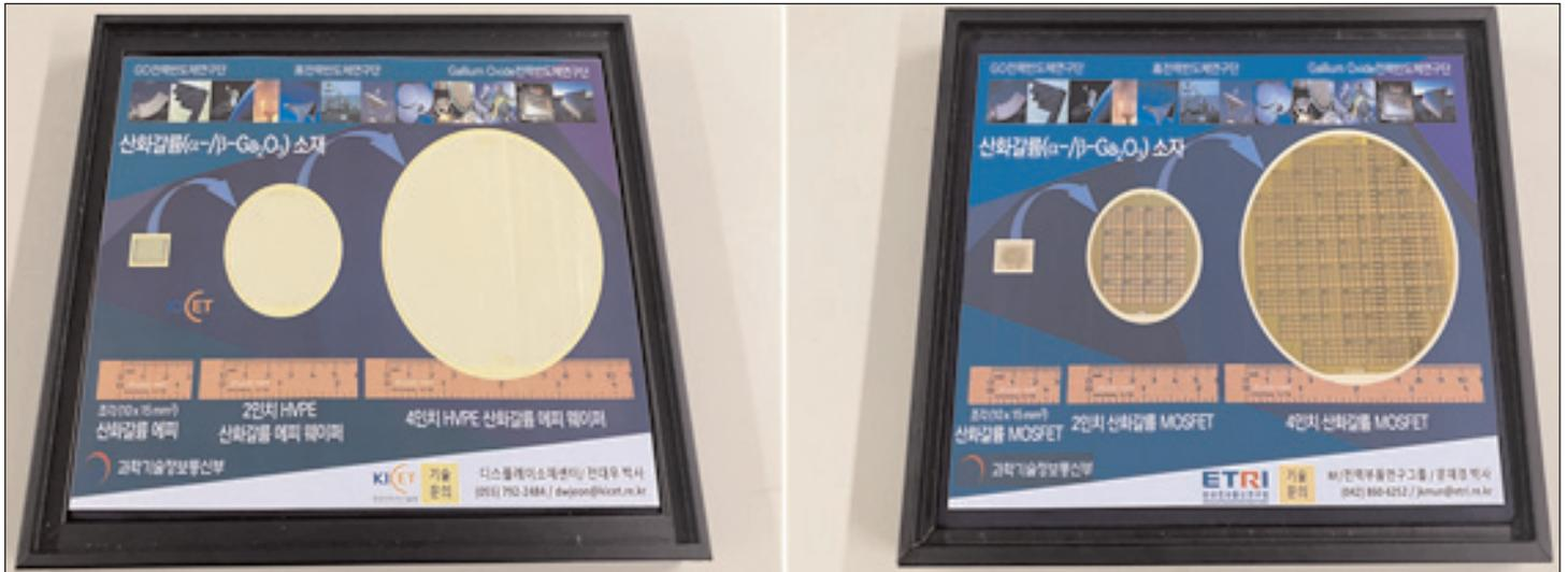
**Gallium oxide epiwafer for high-efficiency power semiconductor (left) and power semiconductor MOSFET (right) (size: piece → 2-inch → 4-inch).**
