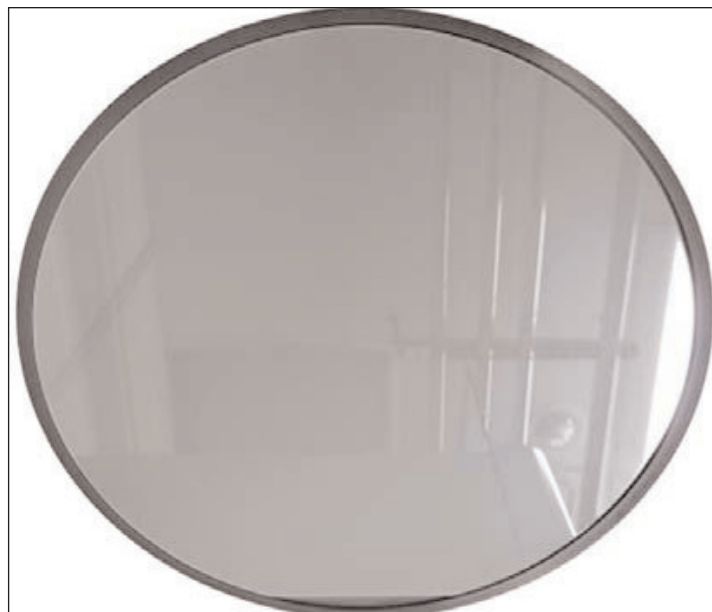
Figure 1. Six-inch GaN template on sapphire substrate fabricated using QF-HVPE system.
