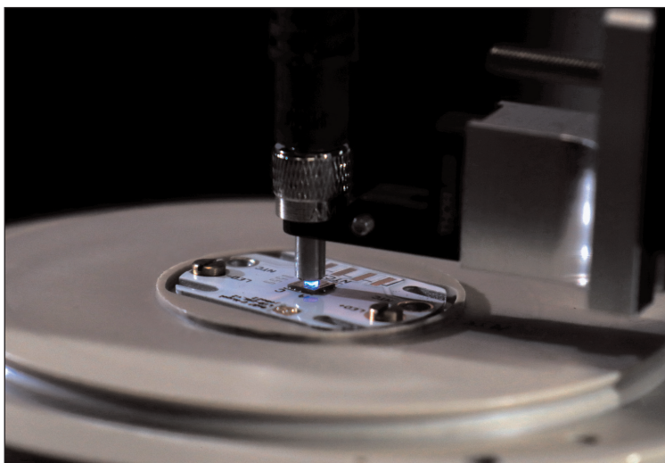
Laboratory setup with far-UVC LED chip consisting of tens of thousands of 235nm micro-LEDs emitting into a glass fiber. © FBH/P. Immerz
