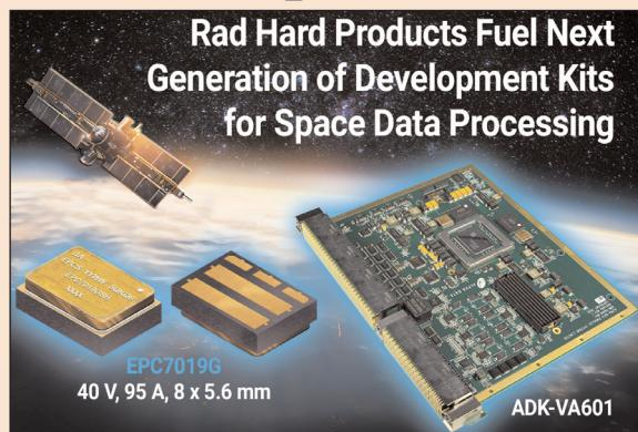
EPC7019G, which is part of EPC Space's latest generation of radiation-hardened devices.
