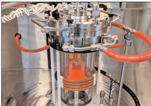
**Heart of the reactor in the MOCVD system. (Image courtesy of Cohen Rautenkranz, Agnitron Technology.)**
