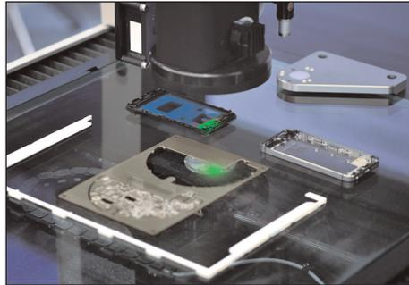
**Green laser offers 4x higher perceived brightness than red lasers traditionally used in industrial equipment.**
