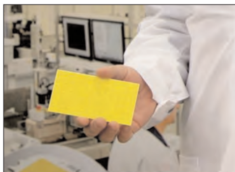
Optogan's X10 LED module consisting of 72 items.
