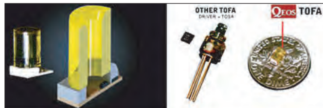
(left) QEOS Transmitter Optical Full Assembly (TOFA). (right) Size of existing optical transmitter compared with QEOS TOFA.
