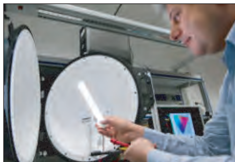
Rifat Hikmet of Philips Research with the first prototype TLED and an integrating sphere.
