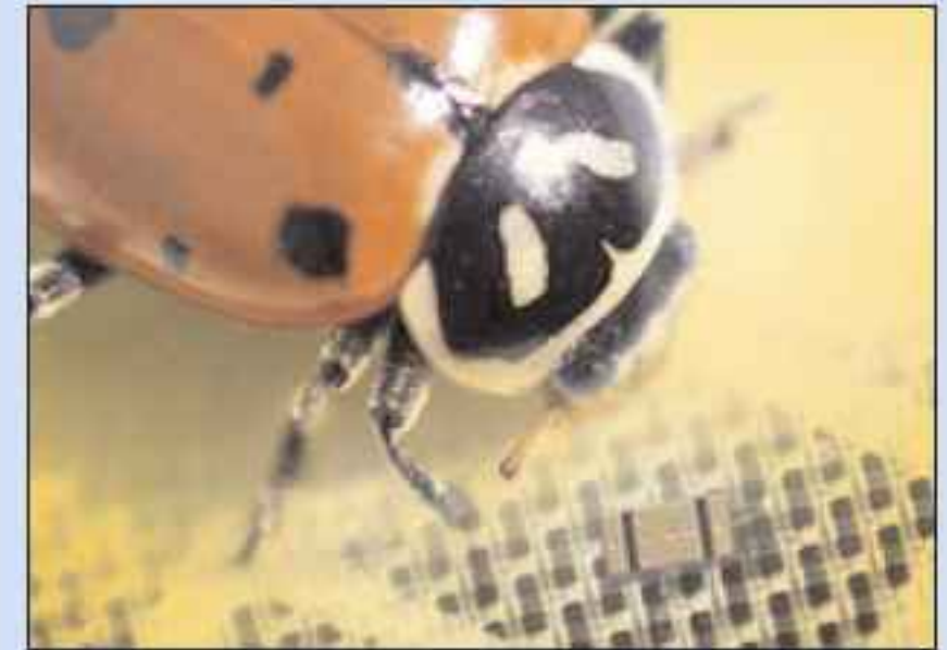
p12 Avago WaferCap 0402-packaged chip uses the first wafer-level chip-scale package (CSP) for RF devices.
