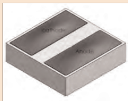
Large p and n bond pads improve Flip Chip packaging reliability.
