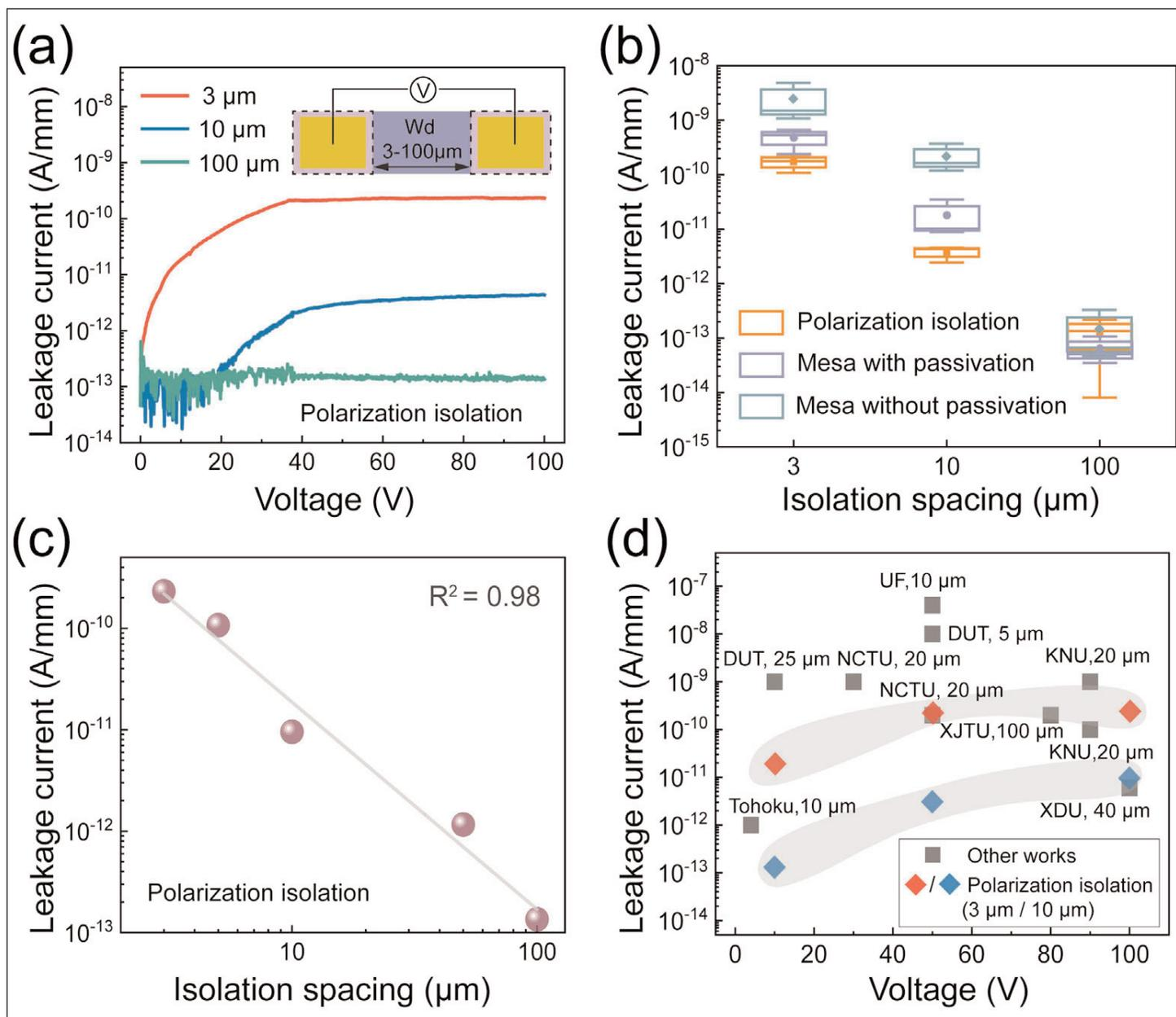
**Figure 2. (a) Leakage versus voltage for PI-HEMT structures. (b) Comparison of PI- with mesa-isolated III-polar HEMT structures with various isolation spacings at 100V bias; (c) leakage versus isolation spacing of PI-HEMT at 100V bias. (d) Benchmarking of leakage versus voltage against state-of-the-art results.**
