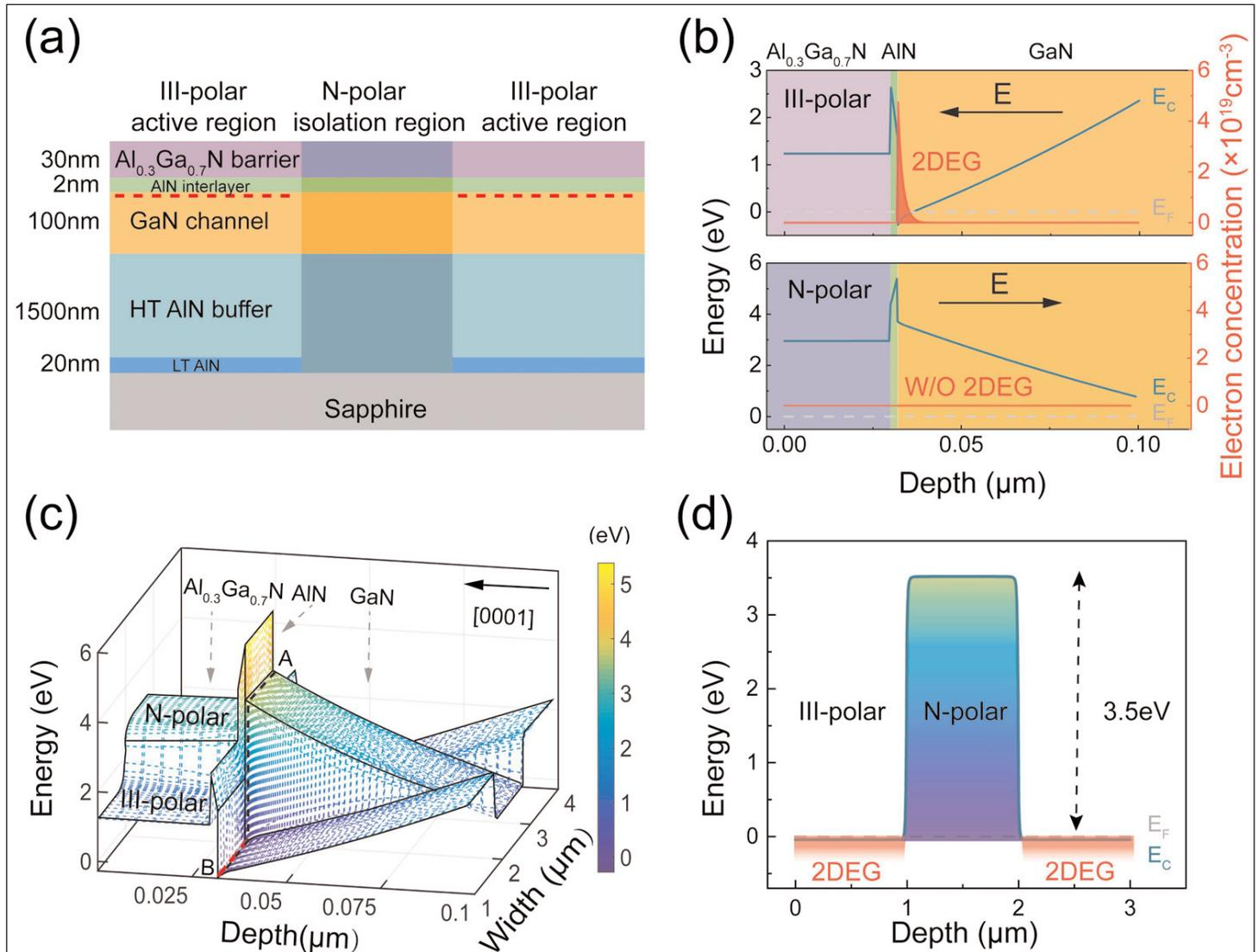
**Figure 1. (a) Cross-sectional PI-HEMT scheme. Red dashed line represents 2DEG. (b) Band diagrams. (c) Three-dimensional mapping of conduction band showing barrier height between III- and N-polar GaN of PI-HEMT structure with  $1\mu\text{m}$  N-polar width (i.e. isolation spacing). (d) Conduction band diagram extracted from dashed line A-B in (c).**
