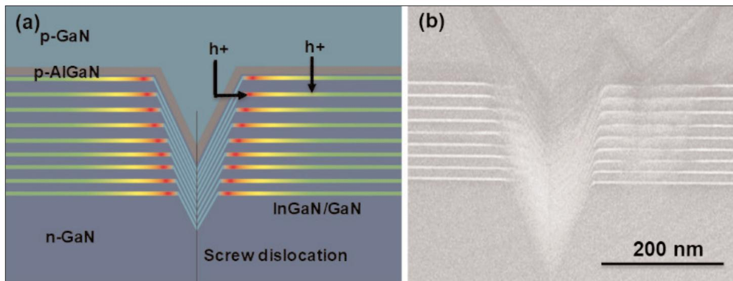
**Figure 1. (a) Schematic of V-groove in color-tunable LEDs showing varying indium content and hole injection pathways, (b) transmission electron micrograph of grown structure showing V-groove.**
