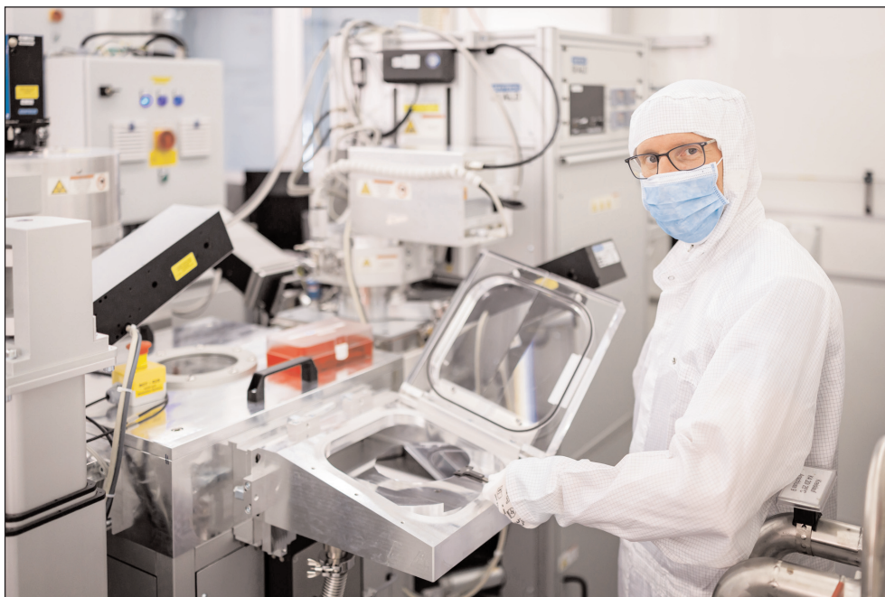
Researcher at Fraunhofer THM inserting a wafer into the transfer chamber of a deposition/etching cluster for structuring using atomic layer etching. © Daniel Karmann/Fraunhofer IISB.
