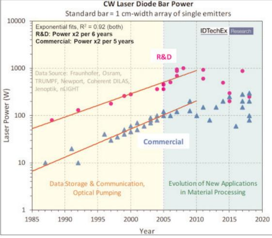
applications of laser The increase in diode bar power contributed to the development of direct diode lasers diodes include data storage, data communication technology includes the improvement of infrared beam quality for precision engineering and the development of novel visible light lasers for metal processing.
