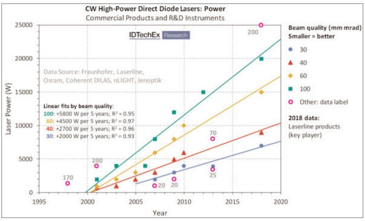
Evolution of output power and beam quality in high-power direct diode lasers (HPDDLs) at 1 $\mu$ m infrared wavelength, according to data collected and analysed by IDTechEx. HPDDLs are a rapidly evolving tool for material processing and industrial manufacturing.
