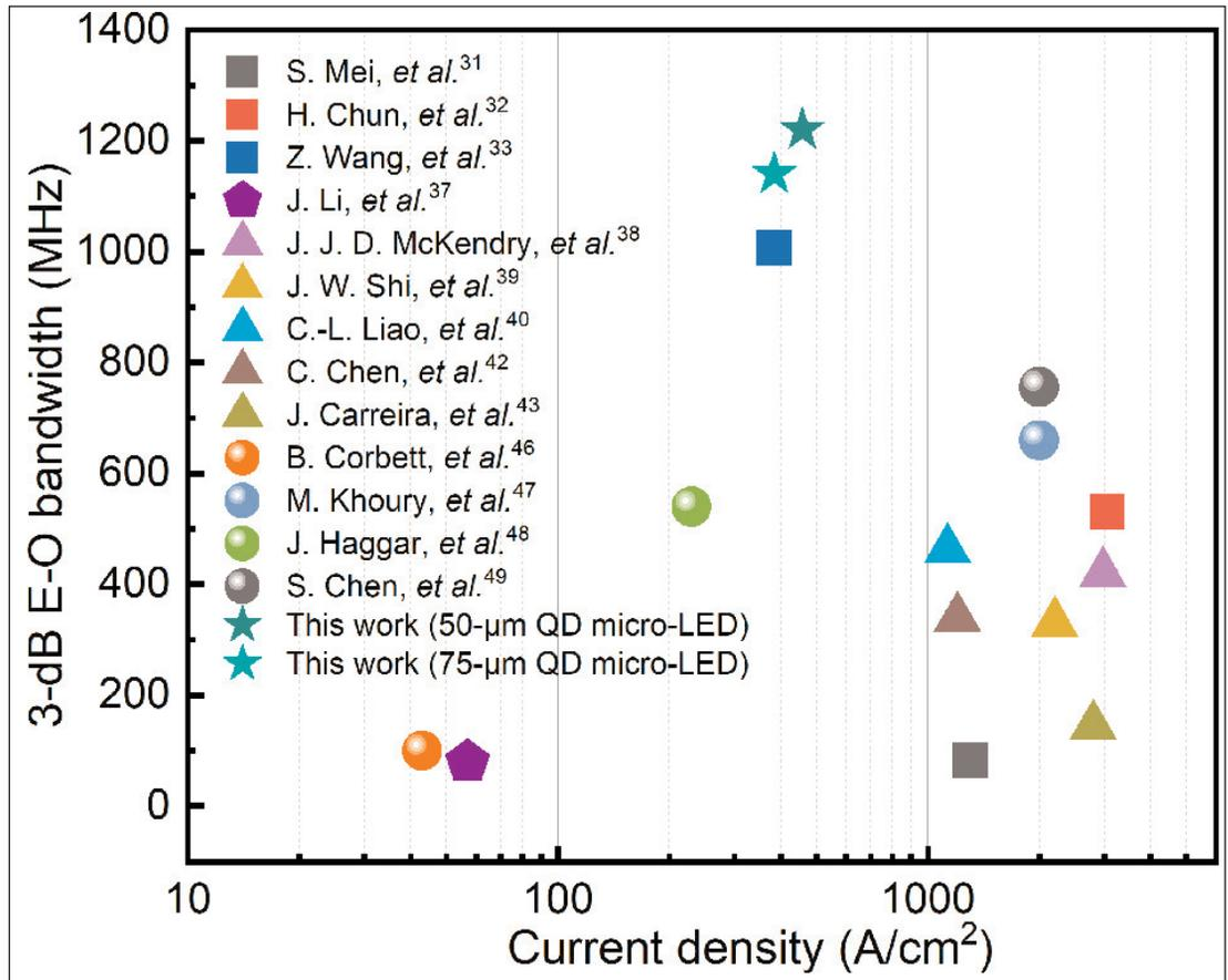
**Figure 2. Benchmarks of 3dB E-O bandwidth of long-wavelength LEDs versus various current densities (square symbol: white-light LED; pentagon symbol: surface plasmon-coupled LED; triangle symbol: c-plane LED; sphere symbol: semipolar green LED; star symbol: QD green micro-LED in work reported here).**
