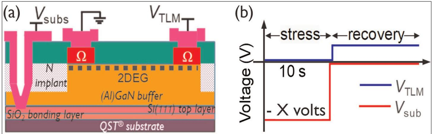
**Figure 2. (a) Test structure and (b) test procedure to measure buffer dispersion. X varies from -650V to -1200V, depending on stack thickness.**
