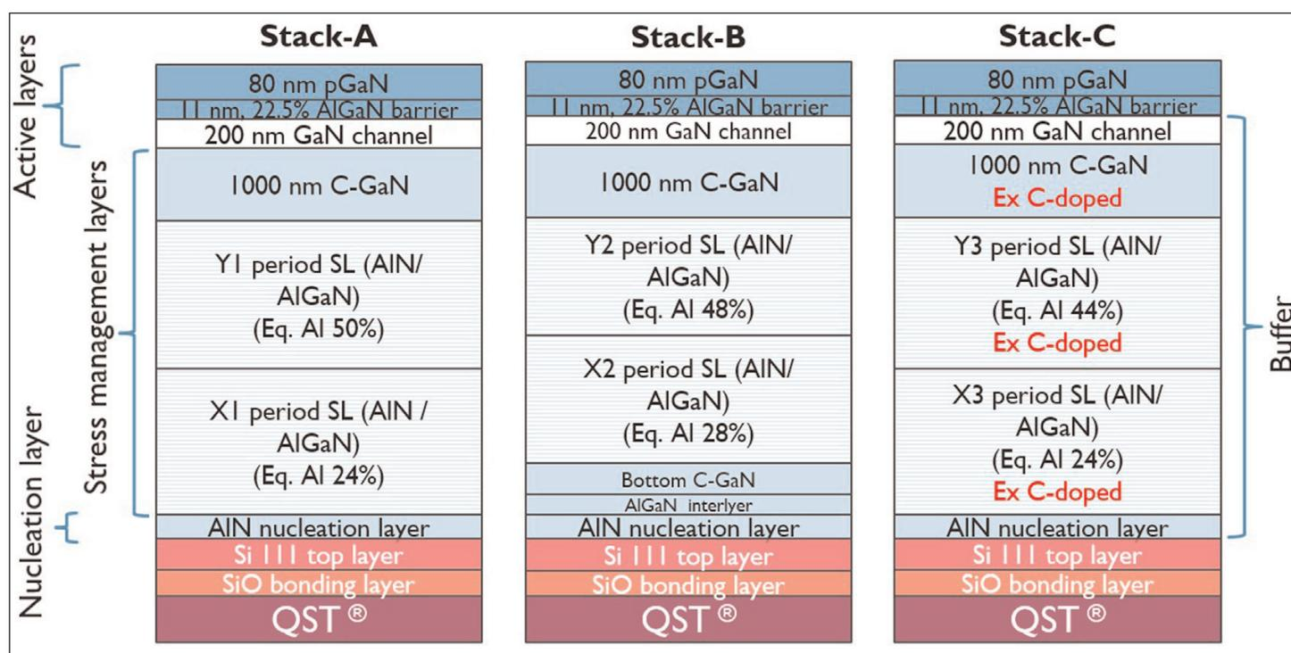
**Figure 1. High-electron-mobility transistor (HEMT) stacks based on intrinsic (stack A and stack B) and extrinsic (stack C) C-doping. Buffer thicknesses of stack A and stack B varied from 5.3–7.4µm to 4.8–6.1µm, respectively. Stack C had a thickness of 6.8µm.**
