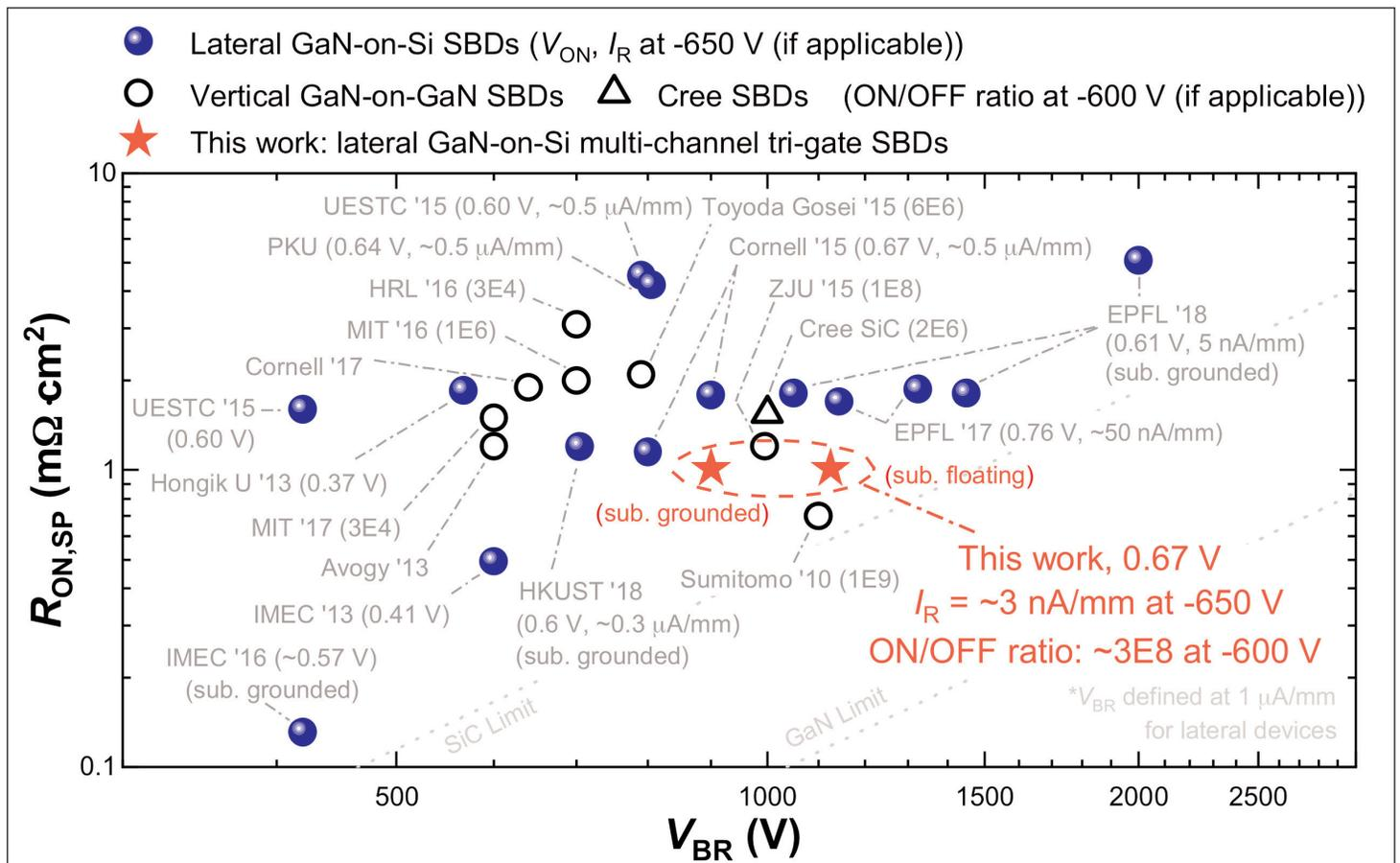
**Figure 4. Specific on-resistance ( $R_{ON,SP}$ ) versus  $V_{BR}$  benchmark of multi-channel tri-gate SBDs against state-of-the-art lateral GaN SBDs. Some values were recalculated for fair comparison.**
