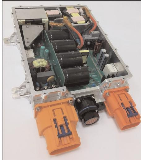
hybrid vehicles/electric vehicles (PHEV/EV) applications. With a universal 110–220V/16–32A AC input and 200–430V DC output for charging the automotive battery by controlling voltage and current flow to the battery, the charger is
