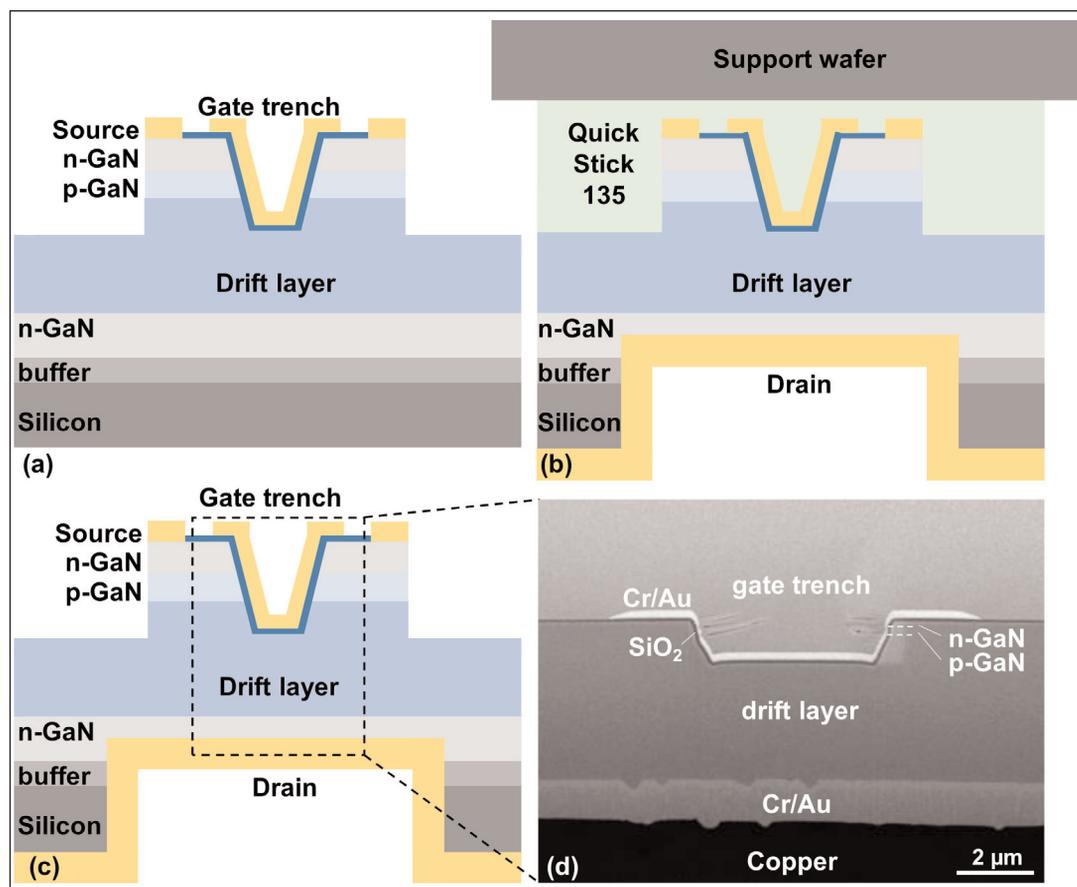
**Figure 1. (a) Schematic of device structure after definition of source and gate pads. (b) Drain contact defined at back-side via support wafer attached using QuickStick 135 wax. (c) Schematic of completed device after removing support wafer. (d) Cross-sectional scanning electron microscope image of fabricated fully vertical GaN-on-Si MOSFET.**
