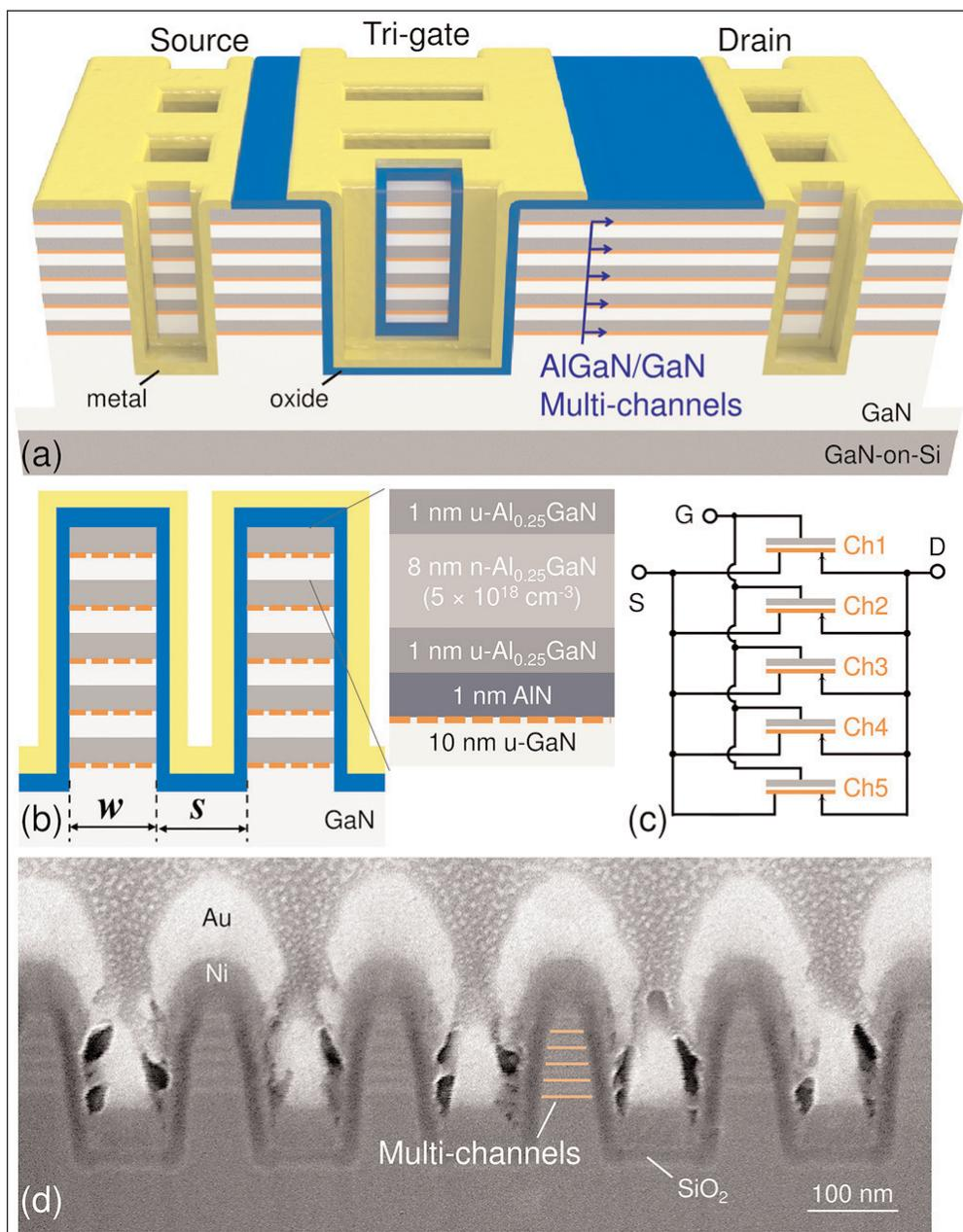
**Figure 1. (a) Schematic of multi-channel tri-gate AlGaN/GaN MOSHEMT. (b) Cross-sectional schematic of tri-gate region. Inset shows multi-channel heterostructure. (c) Equivalent circuit. (d) Cross-sectional scanning electron microscope image of tri-gate region, tilted by  $52^\circ$ .**
