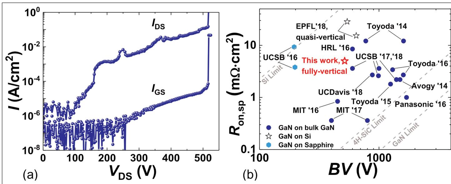
**Figure 2. (a) Off-state blocking performance of metal mask vertical MOSFET measured at 0V gate potential. (b)  $R_{on,sp}$  versus BV benchmarking against other reported GaN vertical transistors on bulk GaN and Si substrates.**
