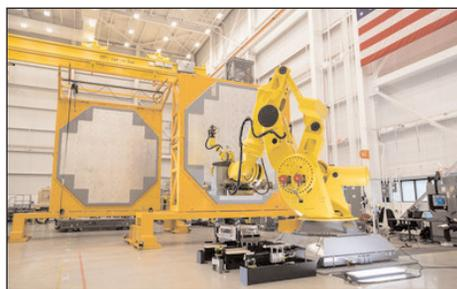
AN/SPY-6(V) is the US Navy's next-generation integrated air and missile defense radar. Currently in production and on track for the DDG-51 Flight III destroyer, SPY-6 employs gallium nitride-based technology to enable 360° active electronically scanned array (AESA)
