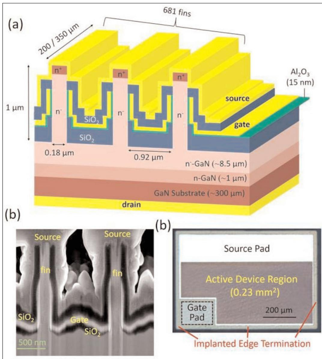
**Figure 5. (a) Three-dimensional schematics of GaN vertical power FinFETs with multiple fin channels. (b) Cross-sectional scanning electron microscope (SEM) image of fin area, taken in focused ion beam system. (c) Optical microscope image.**
