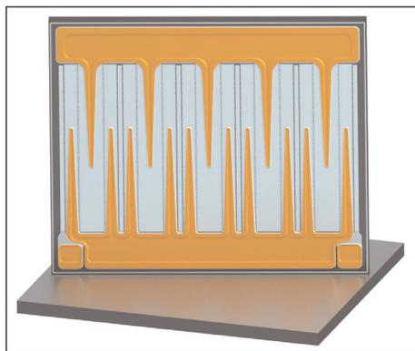
**GaN Systems' new GS-065-080-1-D 80A, 650V GaN E-HEMT power transistor.**
