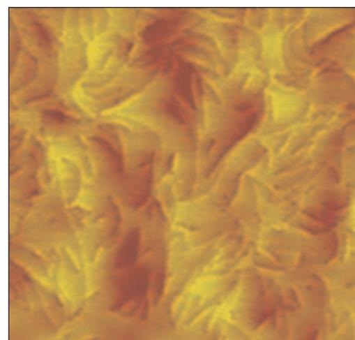
**Figure 1: Epi structure of IGaN's GaN-on-Si epi for power applications.**
