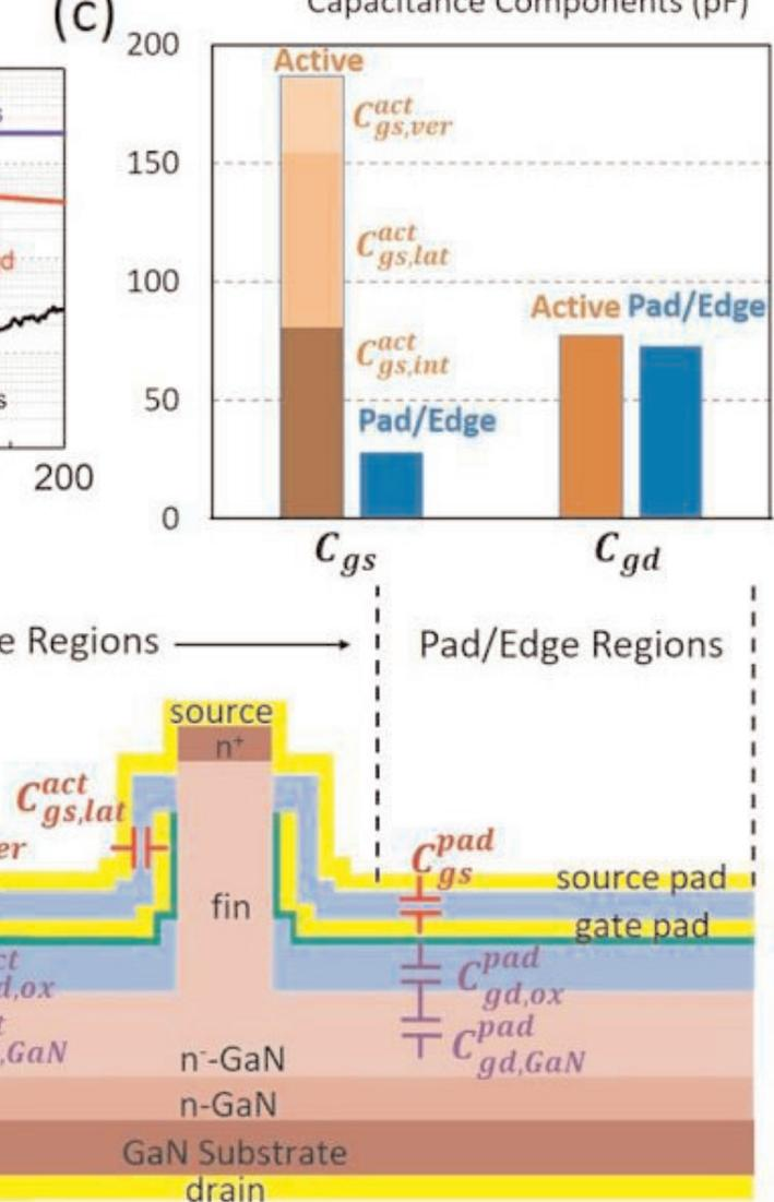
**Figure 6. (a) Device junction capacitances  $C_{ds}$ ,  $C_{gs}$  and  $C_{gd}$  measured by using Agilent B1505A power device analyzer and custom-built RC circuit. (b) Schematics of different  $C_{gs}$  and  $C_{gd}$  components in active and pad/edge regions. (c) Calculated components break-out for measured  $C_{gs}$  and  $C_{gd}$ .**
