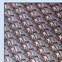
Cover: A processed gallium nitride (GaN) wafer, as used by Fraunhofer-IAF to grow lattice-matched ScAlN for high-voltage, high-current transistors. GaN and AlGaN is now also being grown with fin structures for multi-channel and vertical-current-flow devices in high-power electronics. **p62**
