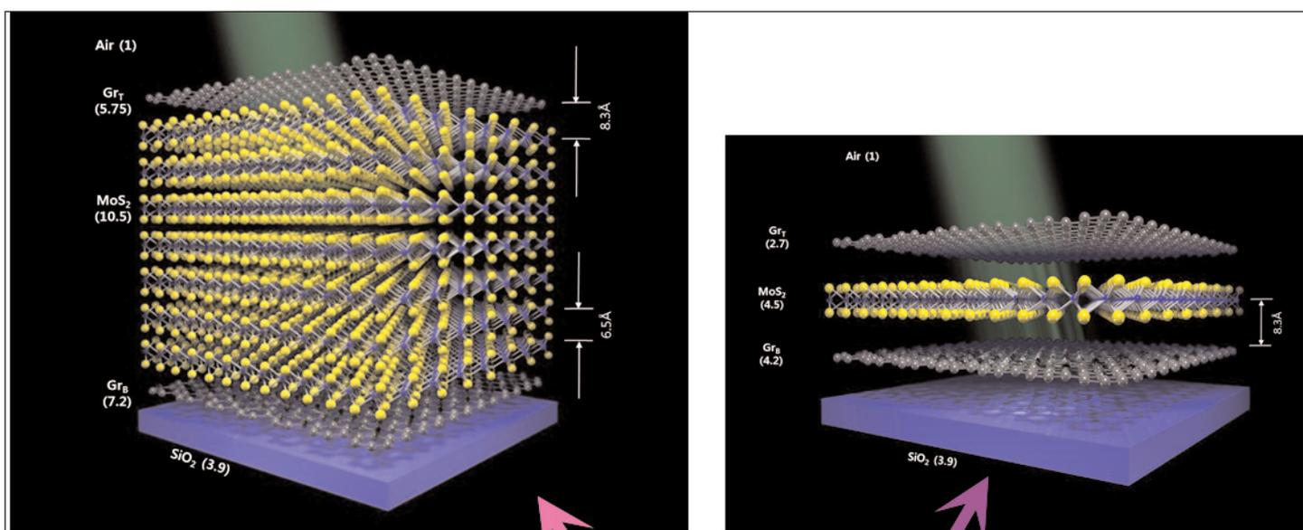
(top) Devices with one-layer and seven-layer MoS<sub>2</sub> were built on top of a silicon base and compared. Dielectric constants responsible for the difference in electrostatic potentials are shown in parenthesis.
