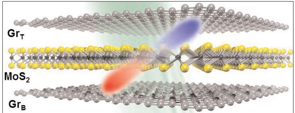
**Device with MoS<sub>2</sub> layer sandwiched between top (GrT) and bottom (GrB) graphene layers. Light (green ray) is absorbed and converted into electric current. When light is absorbed by the device, electrons (blue) jump into a higher energy state and holes (red) are generated in the MoS<sub>2</sub> layer. Motion of holes and electrons created by the difference in electronic potential between the GrT-MoS<sub>2</sub> and the GrB-MoS<sub>2</sub> junctions generates the electric current.**
