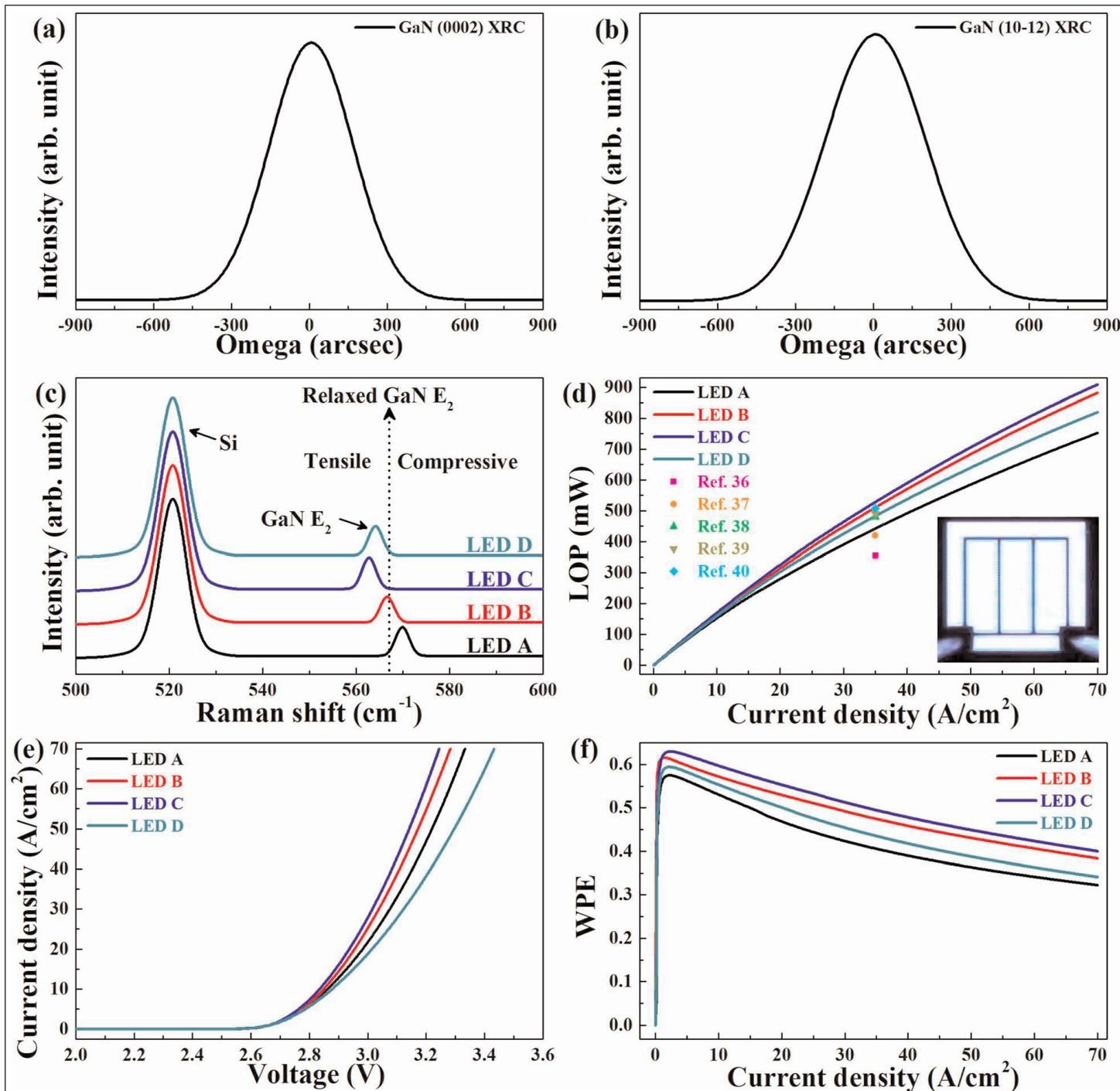
**Figure 2. (a) GaN(0002) and (b) GaN(10 $\bar{1}2$ ) XRCs for LED C, (c) Raman spectra of LEDs A to D. (d) Experimental light output power versus current density, (e) current density versus voltage, and (f) wall-plug efficiency versus current density for LEDs A to D.**
