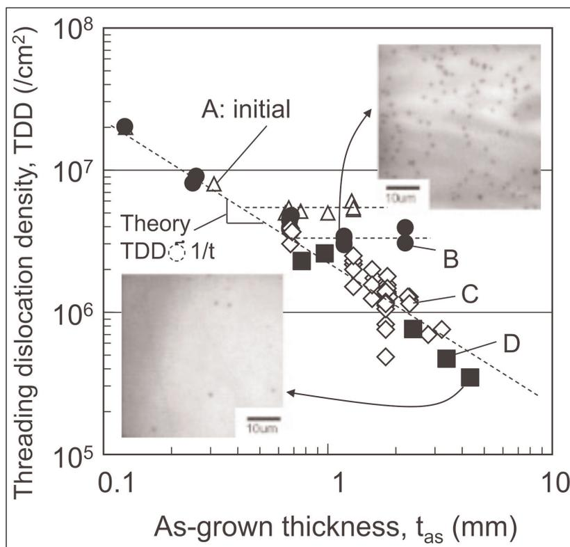
**Figure 5. Relationships between as-grown thickness ( $t_{\text{as}}$ ) and TDD for macro-defect-free GaN substrates grown by VAS method using conditions A–D. Insets: cathodoluminescence (CL) images for GaN substrates grown using conditions B and D.**
