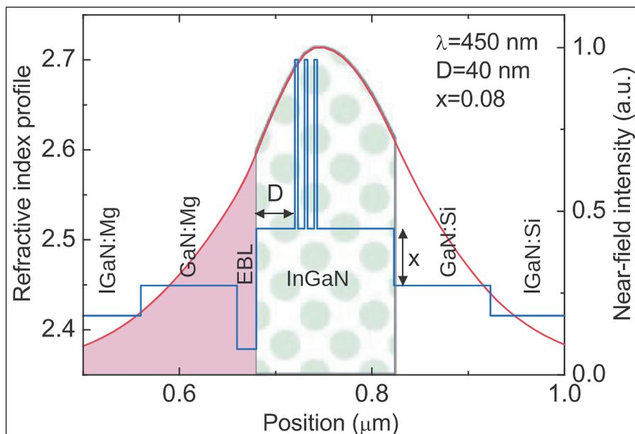
**Figure 3. Refractive index profile and corresponding optical mode distribution of blue LD. Solid purple and dotted green regions correspond to optical mode confined within Mg-doped region and InGaN waveguide, respectively.**
