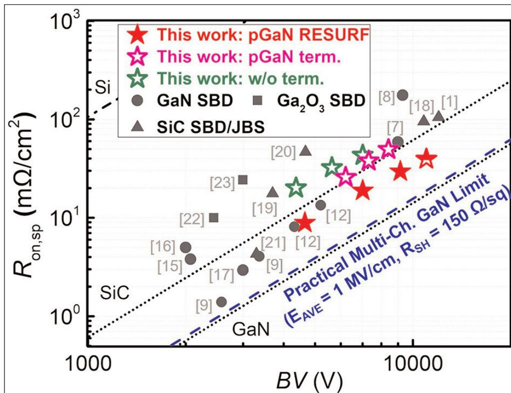
**Figure 2. Differential  $R_{ON,SP}$  versus BV benchmarks for the presented SBDs and state-of-the-art GaN, SiC, and gallium oxide ( $\text{Ga}_2\text{O}_3$ ) high-voltage SBDs. Dotted lines show indicated theoretical limits.**
