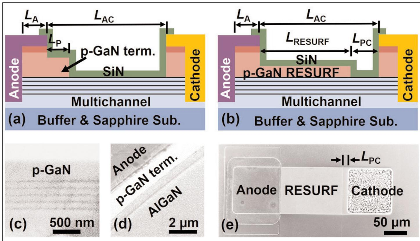
Figure 1. Schematics of multi-channel AlGaN/GaN SBD with (a) p-GaN edge termination and (b) p-GaN RESURF. Cross-sectional scanning electron microscope images of (b) p-GaN/multi-channel region, (c) p-GaN edge termination region, (d) top-view of p-GaN RESURF ( $L_{AC} = 123\mu\text{m}$ ) before SiN<sub>x</sub> passivation.
