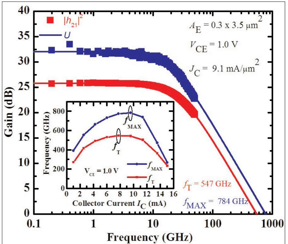
**Figure 1.** Short-circuit current gain ( $|h_{21}|^2$ ) and Mason's unilateral gain ( $U$ ) measured between 0.2GHz and 50GHz. Inset dependence of  $f_T$  and  $f_{\text{MAX}}$  on collector current at 1.0V  $V_{\text{CE}}$ .
