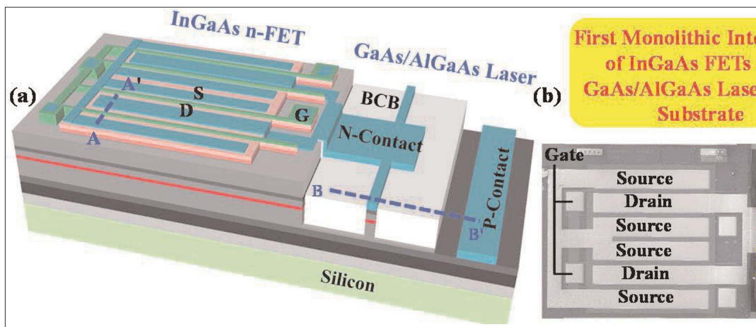
**Figure 1.** (a) Three-dimensional schematic of monolithic integration of InGaAs n-FETs with lasers on silicon substrate. (b) Cross-sectional schematic along A-A' in (a). (c) Cross-sectional schematic along B-B' in (a). (d) Cross-sectional schematic of the laser structure.
