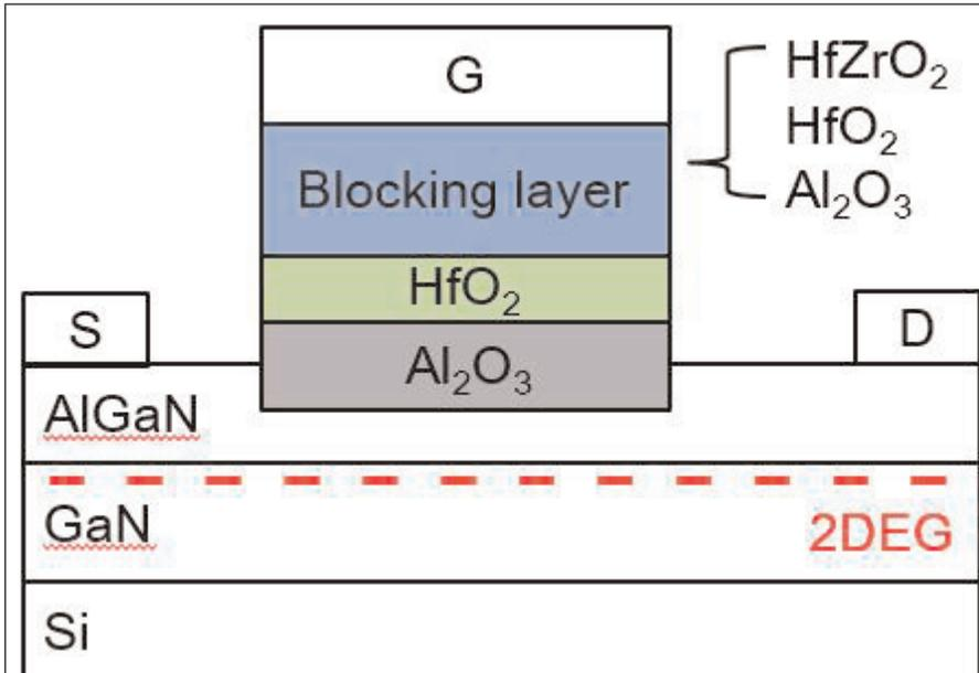
**Figure 6. Schematic cross section of GaN MIS-HEMT.**
