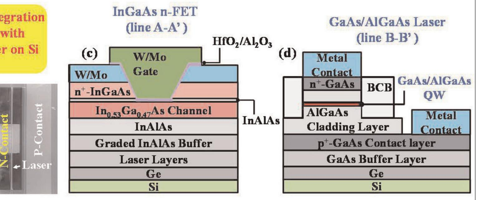
Figure 1. (a) Top-view scanning electron microscope (SEM) image of optoelectronic integrated circuit with multiple laser diodes. (b) Top-view SEM image of optoelectronic integrated circuit with multiple laser diodes. (c) Cross-sectional view of the InGaAs n-FET. (d) Cross-sectional view of the GaAs/AlGaAs Laser.
