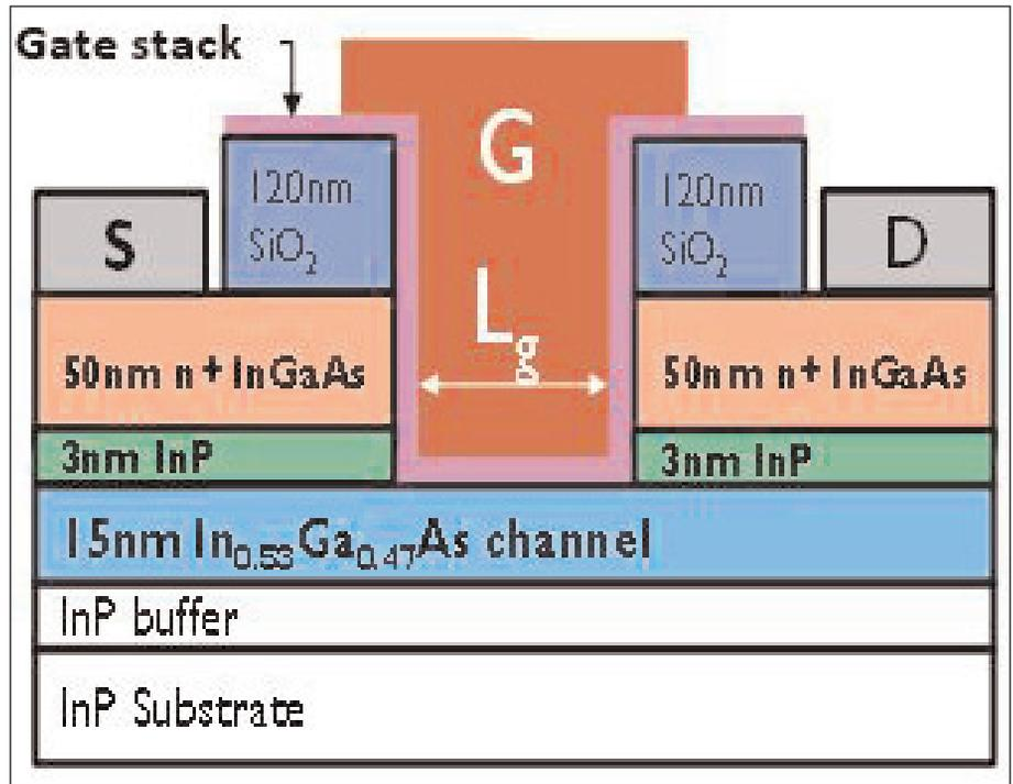
Figure 4. Implant-free InGaAs n-MOSFET.
