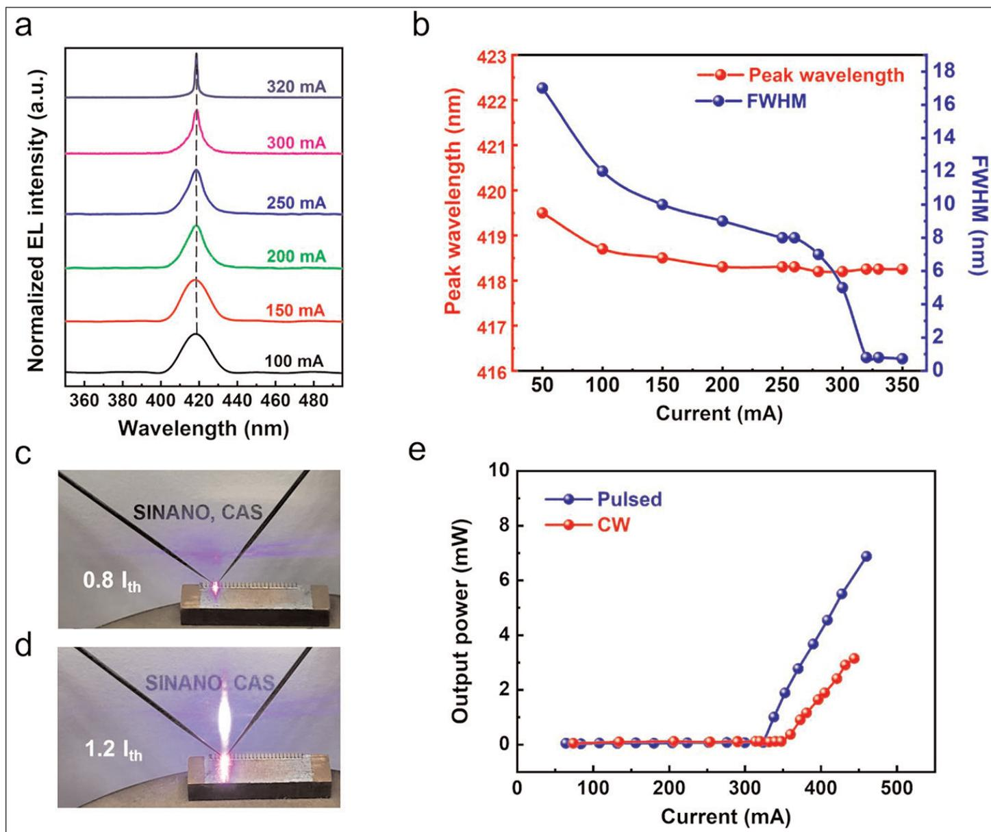
**Figure 3. Electroluminescence of nRW-LD under electrical injection. (a) Spectra under pulsed currents (0.4% duty cycle, 10kHz repetition rate) at room temperature (RT). (b) Peak wavelength and FWHM of spectra versus pulsed injection current at RT. (c, d) Far-field patterns observed 0.8x and 1.2x threshold current. (e) Light output power versus pulsed and CW injection current at RT.**
