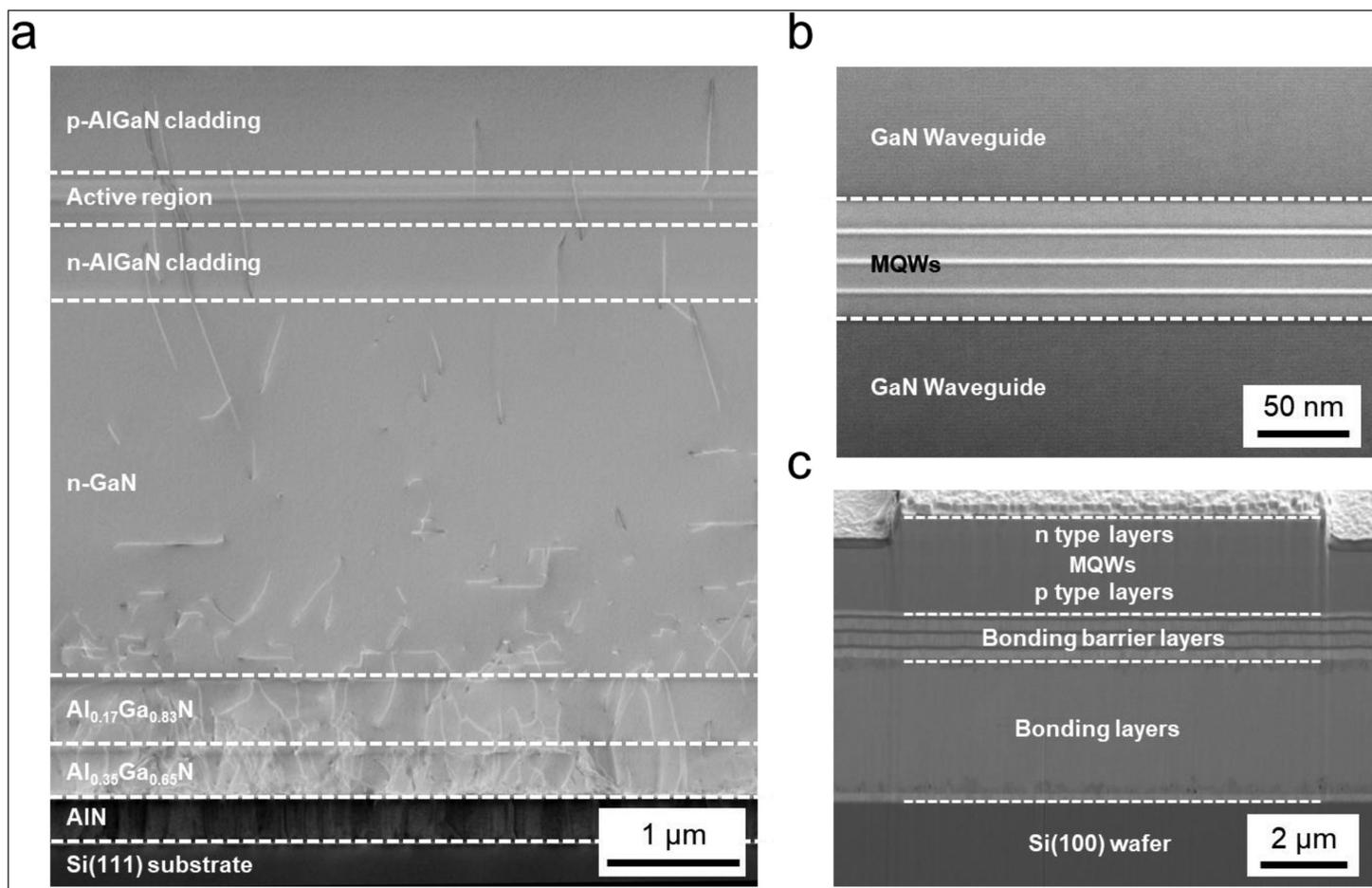
**Figure 1. Cross-sectional images of nRW-LD structures. (a) Scanning transmission electron microscopy of nRW-LD epitaxial structure on Si(111) substrate. (b) Enlarged image of InGaN/GaN quantum wells. (c) Cross-sectional scanning electron micrograph of device bonded to Si(100) wafer.**
