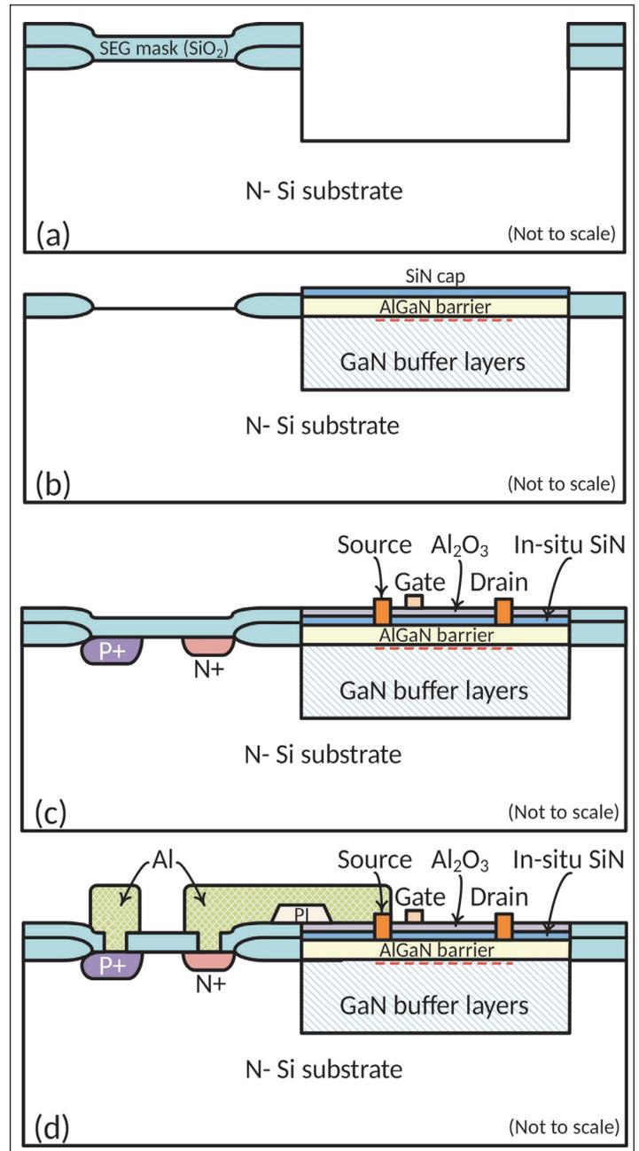
**Figure 2. Schematic cross sections: (a) after recessed window formation, (b) after AlGaIn/GaN epitaxial structure growth, (c) after Si and GaN fabrication, (d) after metal-line interconnection deposition.**
