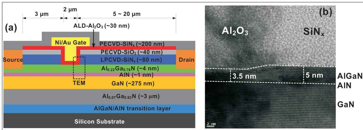
**Figure 3. (a) Schematic device structure of normally-off  $\text{Al}_2\text{O}_3/\text{AlGaN}/\text{GaN}$  MIS-HEMTs fabricated on UTB  $\text{AlGaN}/\text{GaN}$  heterostructures. (b) Transmission electron microscope cross-sectional view of device's gate corner.**
