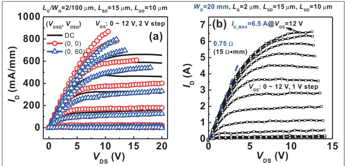
**Figure 4. (a) Pulsed drain current ( $I_D$ ) versus drain bias ( $V_{DS}$ ) characteristics of fabricated normally-off  $\text{Al}_2\text{O}_3/\text{AlGaIn}/\text{GaN}$  MIS-HEMTs from various quiescent gate, drain bias points ( $V_{GSQ}, V_{DSQ}$ ). (b) Characteristics of fabricated 20mm-gate-width devices.**
