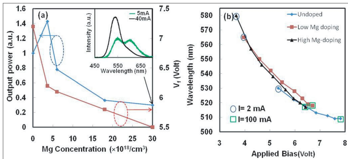
Figure 1. (a) Relative output power and forward voltage ( $V_f$ ) under 20mA injection for LEDs with different Mg doping levels in barrier. The upper right corner shows the electroluminescence (EL) spectra under 5mA and 40mA injection for LEDs with high Mg doping levels (b) EL peak wavelength versus applied bias for current injection levels ranging from 2mA to 100mA for undoped, low-doped ( $3.6 \times 10^{18}/\text{cm}^3$ ), and high-doped ( $1.8 \times 10^{19}/\text{cm}^3$ ) barriers.
