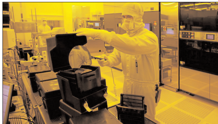
Figure 1: Preparation and processing of SiGe wafers in the IHP pilot line (courtesy R.Weisflog/IHP).
