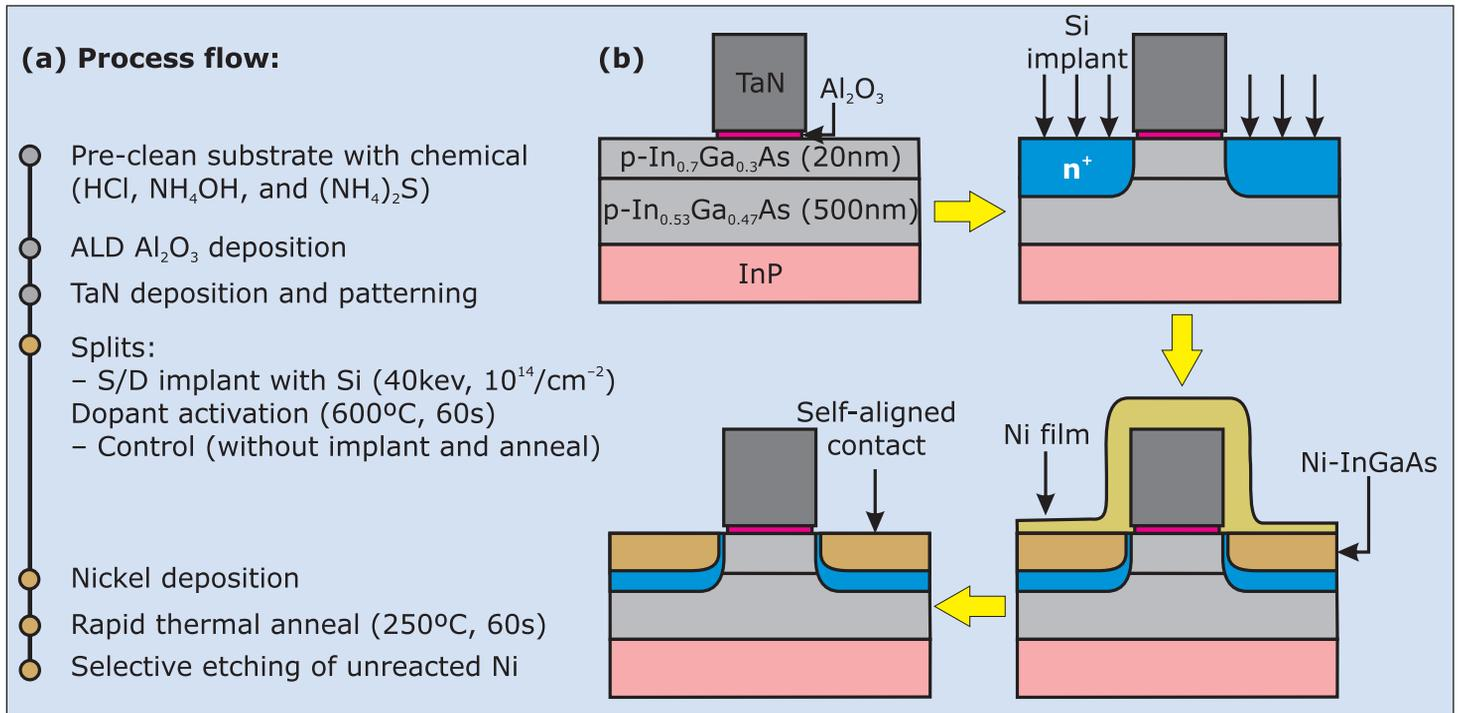
**Figure 1. (a) Process flow for fabrication of In<sub>0.7</sub>Ga<sub>0.3</sub>As n-MOSFETs with self-aligned Ni-InGaAs contacts and metal S/D. (b) The salicide-like metallization process comprises a reaction of Ni with In<sub>x</sub>Ga<sub>1-x</sub>As and a selective removal of excess Ni using a wet etch.**
