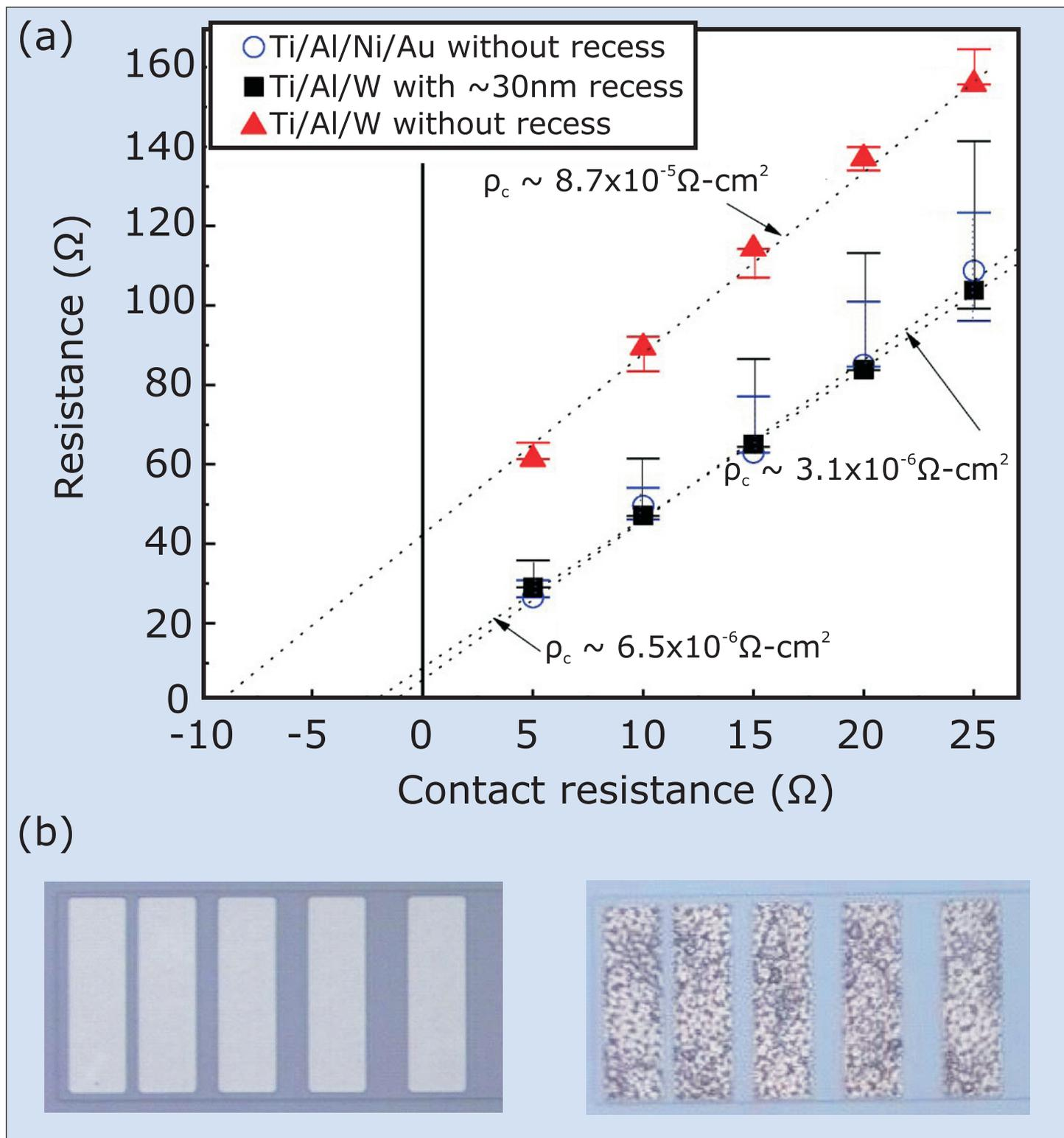
**Figure 5. (a) Total resistance for different ohmic metallization processes as a function of contact distance. (b) Optical micrograph images of the surface for (left) Ti/Al/W recessed contacts and (right) standard Ti/Al/Ni/Au contacts.**
