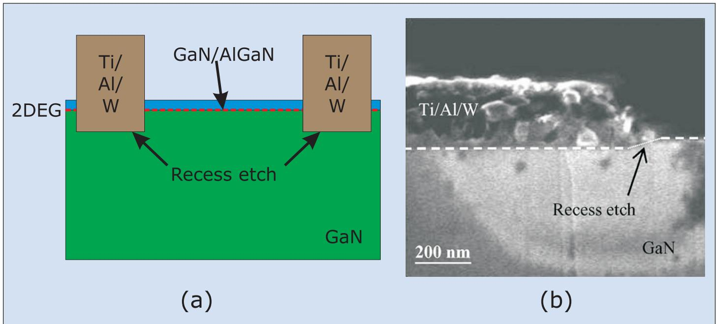
**Figure 4. (a) Schematic cross section of the fabricated undoped AlGaN/GaN HEMTs with S/D ohmic recess. (b) SEM image of the cross section of a Ti/Al/W contact after annealing. Before metallization, the ohmic contact region was recessed  $\sim 30\text{nm}$ .**
