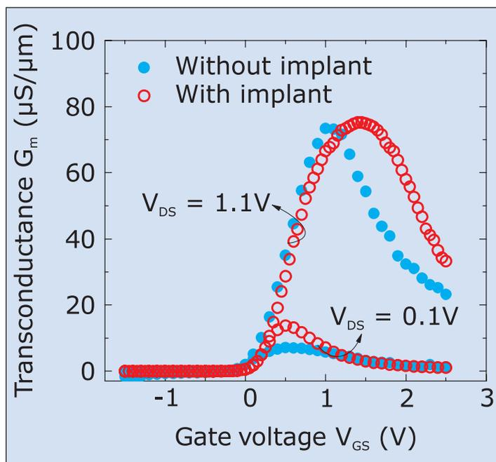
**Figure 3. Transconductance-gate potential ( $G_m$ - $V_{GS}$ ) curves for devices with and without silicon implant of S/D regions. Slight  $G_m$  enhancement was observed for device with S/D implant.**
