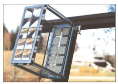
HCPV module with record 41.4% efficiency.
