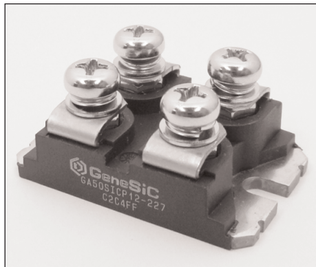
GeneSiC's 1200V/20m \Omega SiC junction transistor-rectifier co-packaged in an isolated SOT-227 package providing separate gate source and sink capability.
