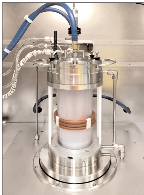
The reactor of Agnitron Agilis 100 MOCVD system can heat substrates up to 1500°C.
