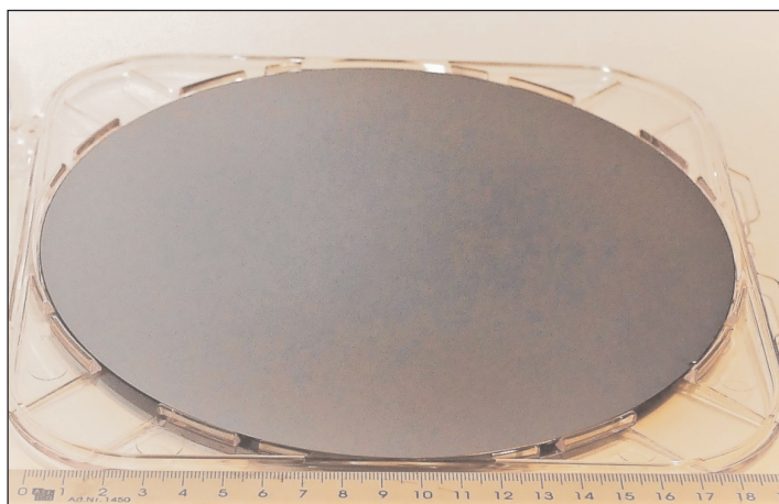
200mm GaN-on-Si epiwafer example for HPE application to be supplied by AZUR based on ALLOS' technology.
