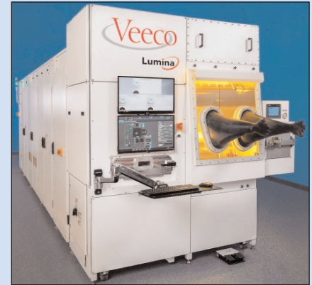
p30 Veeco's new Lumina As/P MOCVD platform, which targets high-volume manufacturing of VCSELs, edge-emitting lasers and mini/micro-LEDs.
