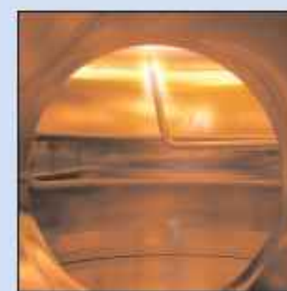
Cover: View inside the patented remote plasma chemical vapour deposition (RPCVD) reactor of Australian firm BluGlass, showing the remote plasma process for fabricating GaN-on-glass blue LED structures, to be demonstrated at the firm's new pilot demonstration plant and headquarters. p36
