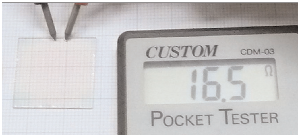
Final SnO 2 thin film grown on glass to make efficient PVs. © 2020 Nakao et al.
