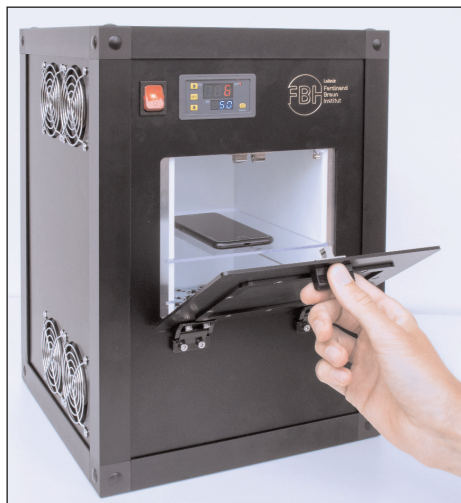
Prototype UVC LED irradiation system to fight multi-drug-resistant pathogens using 120 LEDs - suitable for application to the skin.
