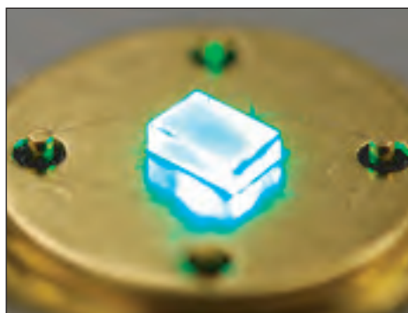
LED chip under test — facet size, 0.3mm x 0.3mm; injection current, 200mA; central wavelength, 525nm.
