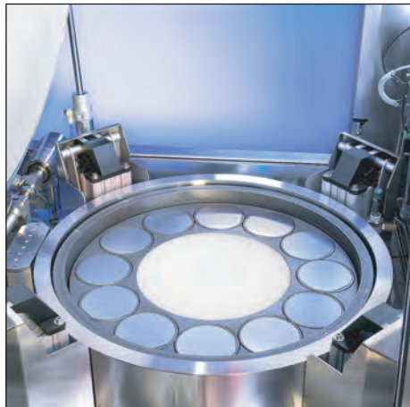
Aixtron's AIX 2600G3 MOCVD planetary reactor for 12x4-, 49x2- or 7x6-inch configurations.
