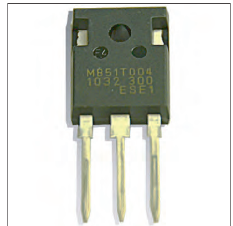
Device prototype in TO247 package.
