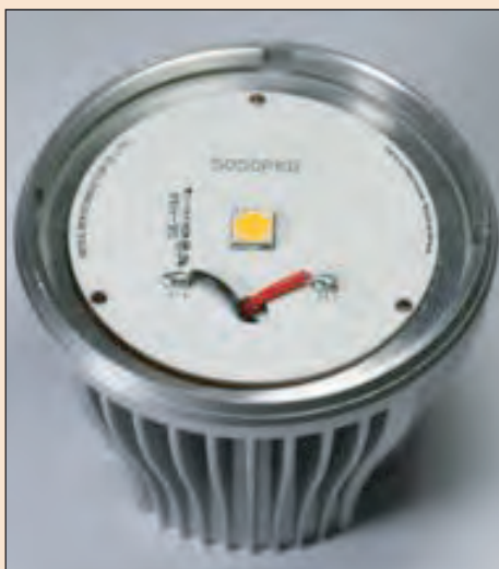
LED bulb using nPola technology requires just one LED.
