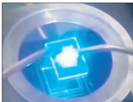
LED chip under light-emitting test: substrate size, 1cm 2 ; chip size, 0.3mm square; injection current, 200mA; center wavelength, 450nm.
