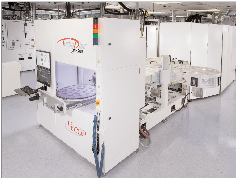
Veeco's TurboDisc EPIK700 GaN MOCVD system for high-volume LED manufacturing.
