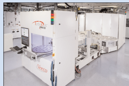
p34 Veeco's new TurboDisc EPIK700 GaN MOCVD system for high-volume LED production, which accommodates 31x4"-, 12x6"- or 6x8"-wafers.
