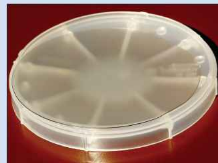
p14 TDI's prototype AlN-based 4" semi-insulating substrate.
