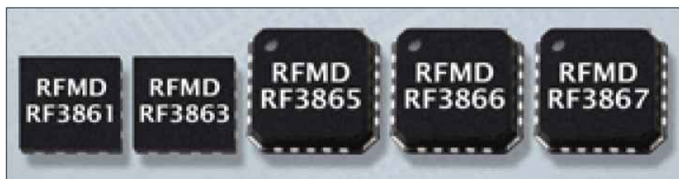
RF Micro Device's new RF386x family GaAs pHEMT low-noise amplifiers.
