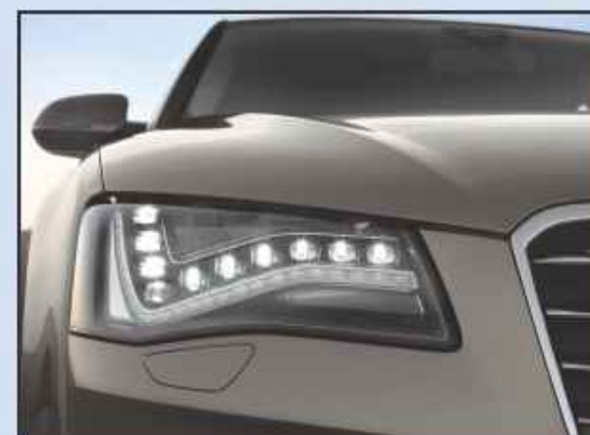
p55 LED light sources in the low-beam lights of the new Audi A8, which uses all-LED Osram headlamps.
