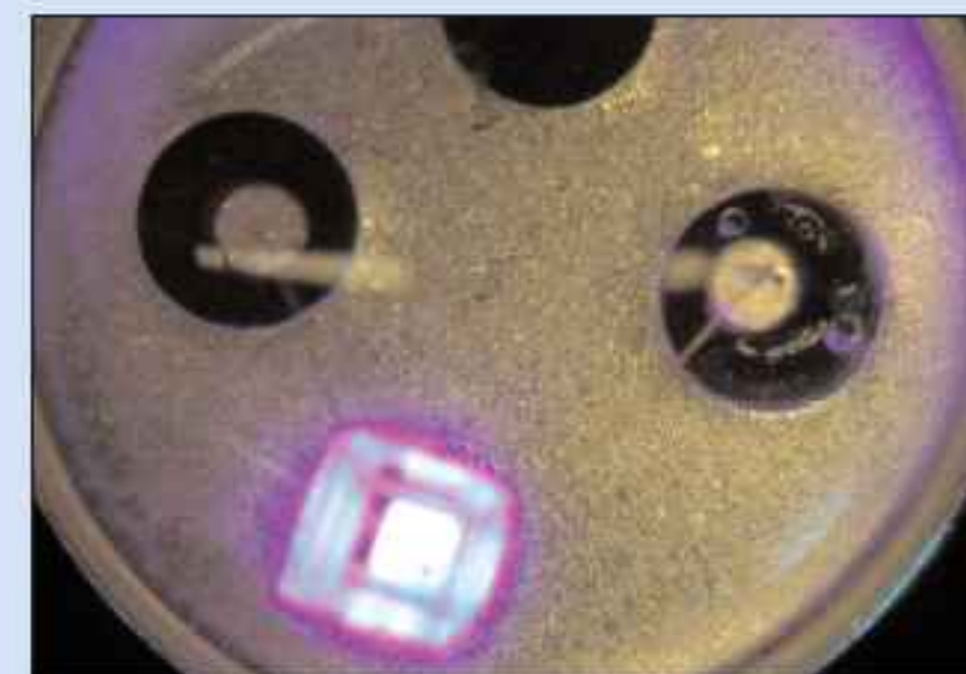
p28 UCSB has used low-defect non-polar m-plane GaN to fabricate LEDs with efficiency of 41% up to 200mA.
