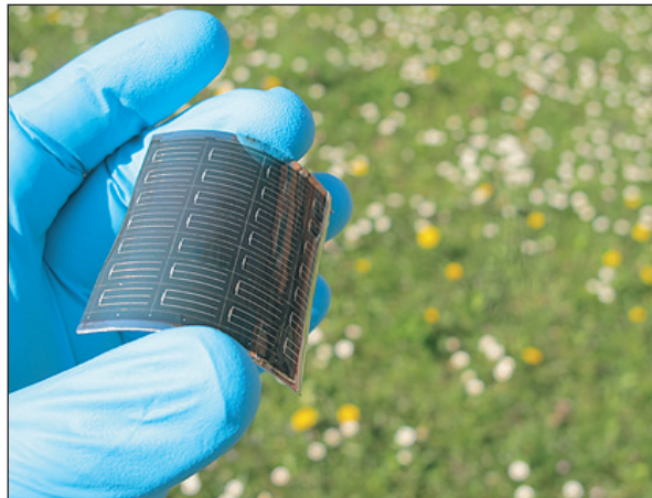
Flexible thin film CIGS solar cell on polymer substrate developed at Empa (Copyright: Empa).
