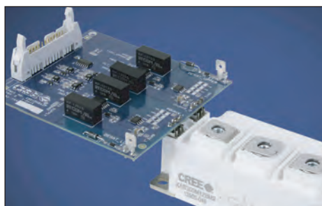
62mm C2M module and direct mount gate driver.
